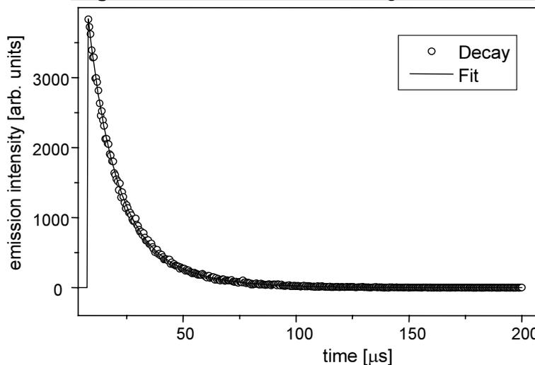
**Fig. 8.** Decay curves for Er<sup>3+</sup> luminescence centres ( $^4S_{3/2} \rightarrow ^4I_{15/2}$  transition,  $\lambda_{\max} = 555$  nm) detected at 295 K (open circles) and the two-exponential fit (solid line).
