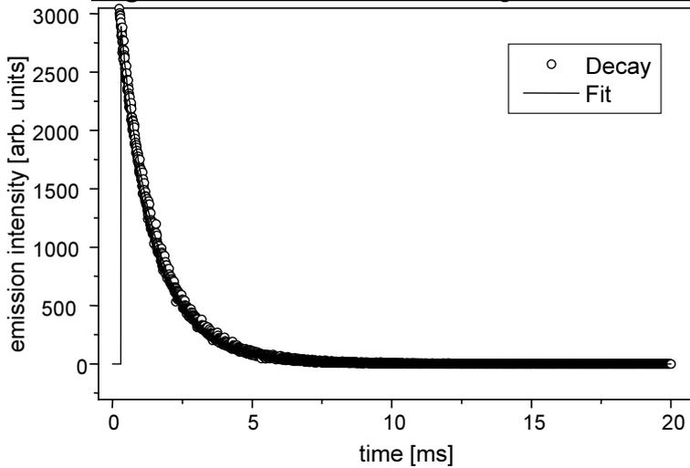
**Fig. 2.** Decay curve for Eu<sup>3+</sup> luminescence centres ( $^5D_0 \Rightarrow ^7F_2$  transition,  $\lambda_{\max} = 615$  nm) detected at 295 K (open circles) and the two-exponential fit (solid line).
