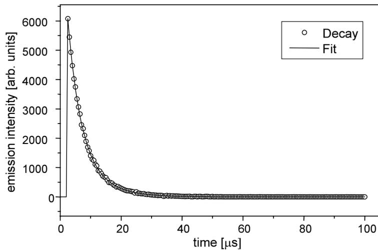
**Fig. 5.** Decay curve for Ho<sup>3+</sup> luminescence centres ( $^5S_2 \rightarrow ^5I_8$  transition,  $\lambda_{\max} = 545$  nm) detected at 295 K (open circles) and the two-exponential fit (solid line).
